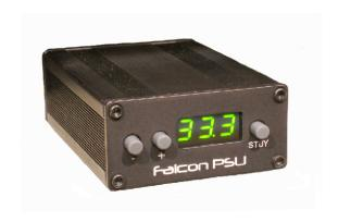
The Falcon Power Supply Unit (PSU) is a microprocessor controlled digital regenerative AC power source used for accurate speed control of a turntable motor. The Falcon will work with any AC Synchronous motor that is 5W or less. The PSU uses Direct Digital Synthesis (DDS) to create an extremely accurate and clean sine wave that improves motor speed stability and allows the user to precisely adjust the turntable platter rotational speed.
